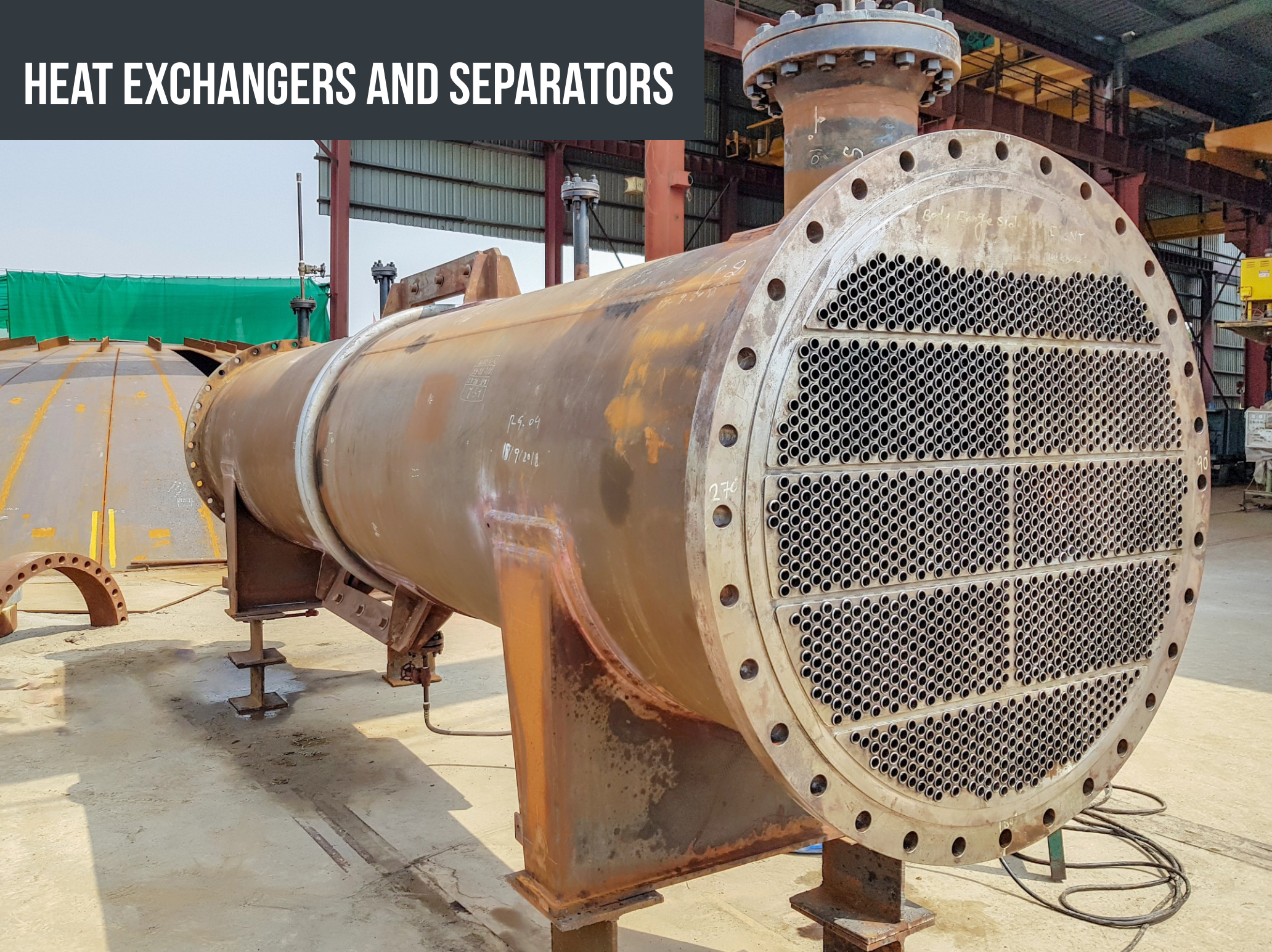
Thermex Heat Exchanger for ICI Pakistan Limited - Polyester plant Type: BEM, Pressure: Shell Side 71 Psig, Tube Side 146.5 Psig, Applicable Code / Standard: ASME Sec. VIII Div. 1 Ed. 2015 & TEMA R 9th Ed.
