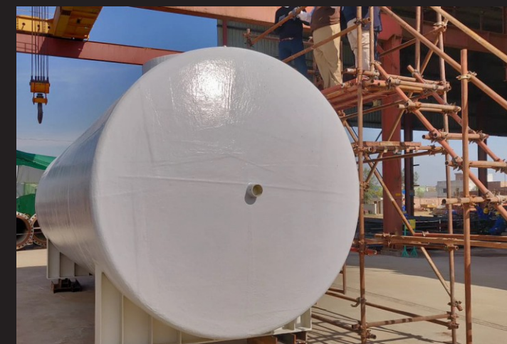
Double Wall Underground Tank manufactured to UL-58 / UL1746 for Total-Parco Pakistan Limited.
