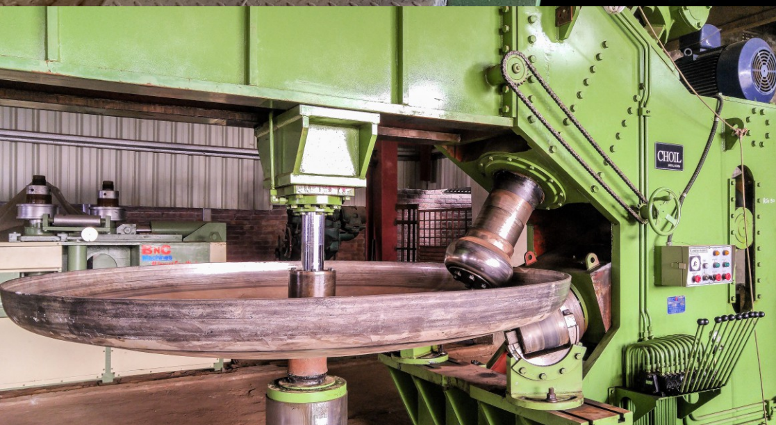
Flanging machine used for forming of dished-ends at Ravi Green Workshop in Lahore, Pakistan.
