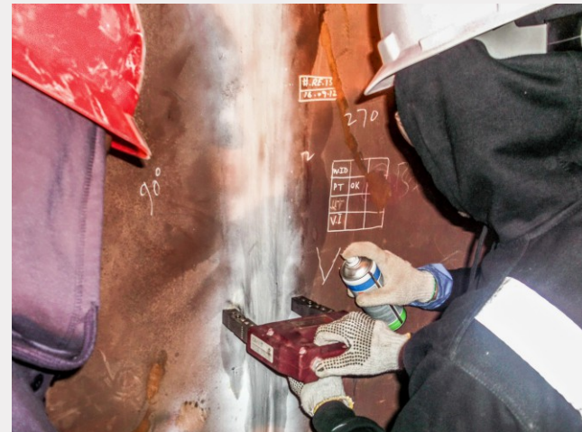
Magnetic Particle Testing (MPT) conducted on the vertical joint of a storage tank.
