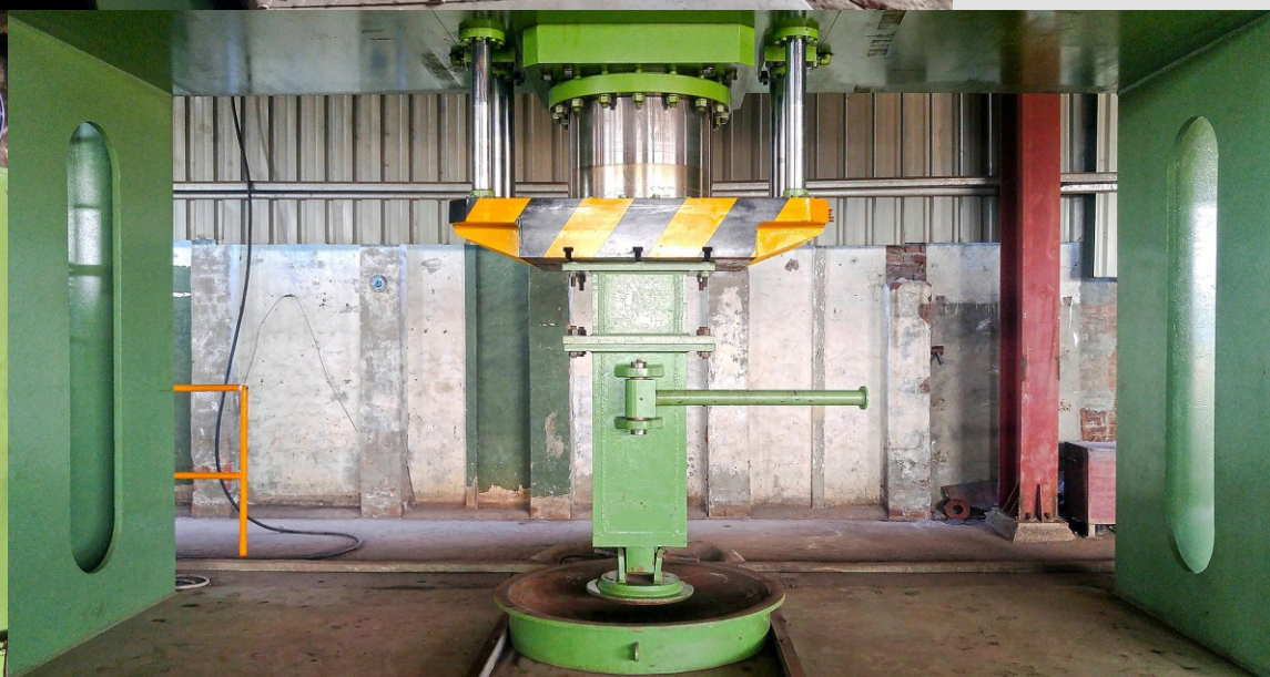
1000 ton force hydraulic press used for dishing of dished-end at Ravi Green Workshop in Lahore, Pakistan.
