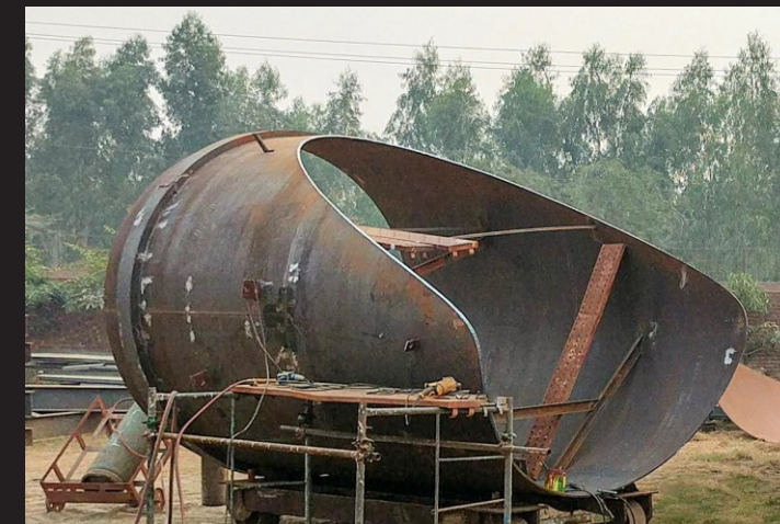
Fabrication of CW Pipe miter cut at 45 degrees for SEPCO-1 Power Plant, Jhang, Pakistan.
