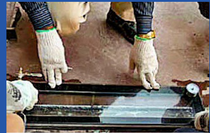
Vacuum box test conducted on the bottom plate joint of a storage tank.
